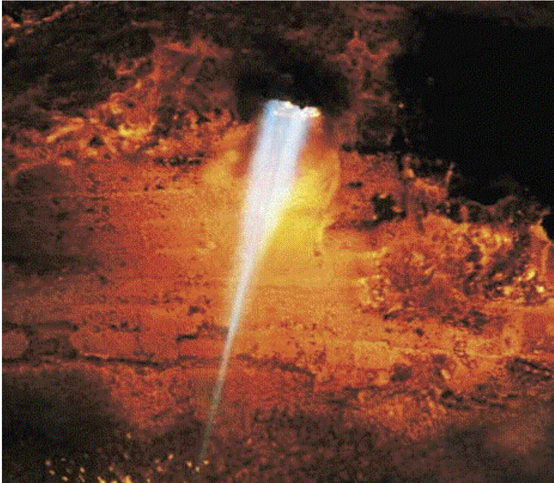
Figure 5. Supersonic Jet Produced by PyreJet Burner
